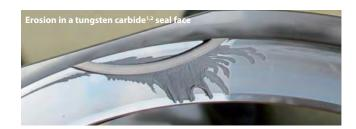
Reactor recirculation pump (RRP) face seals are critical to the safe and efficient operation of nuclear reactors. However, these seals develop electric potential differences (voltage) between the seal faces. This stray voltage drives current across the seal, causing electrical damage to the faces.
