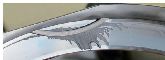
**Fig. 4.** Wide erosion radial canals formed in the tungsten carbide rotating seal face, May 2013.
