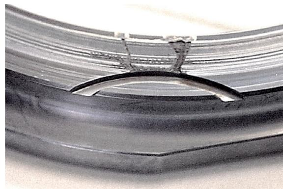
**Fig. 3.** Radial canals in the thermo-hydrodynamic circulation slots, August 2003.
