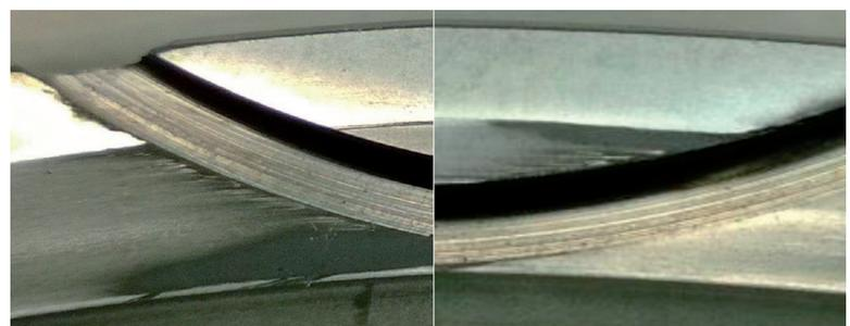
Fig. 5. Tungsten carbide rotating seal face erosion development.
